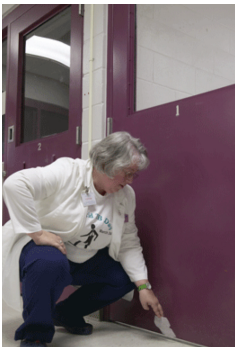
Image 12. Example of a health care worker using a tissue paper to verify negative pressure (Source: Southeastern TB Center)
