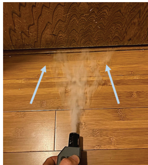
Image 11. Smoke tube testing (Source: Elon Ullman, OHB)
